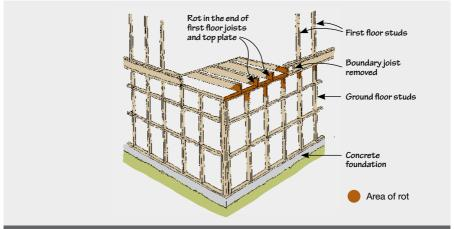
Figure 6a. Rotted ends of first floor joists prior to remediation
