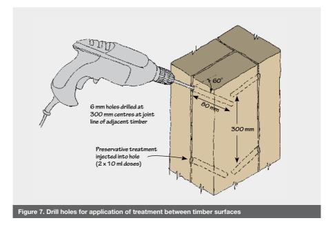
Adhesive tape should be applied to the bottom of the joint before injecting the treatment to minimise treatment running out the bottom of the lintel. One of the main influences on boron coverage is the size of the gap between the two pieces of timber. If the gap is too large, the treatment rapidly runs out with little coverage and penetration. Temporary clamping of the lintel can help minimise this.
