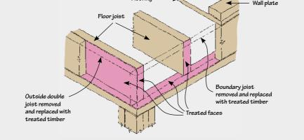
Figure 5. Boundary joist and outer joist removed to apply treatment
