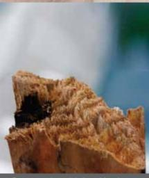
5. Fracture surface of timber with soft rot
